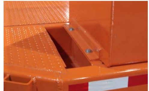
Add rear axel guard if not already in place (this can also be installed at beginning of assembly process).
