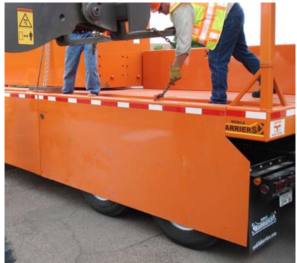
Insert tongue of axel guard through lower corner slot. Pin and clip from inside. Special 7/8" pin is provided. Check that there is adequate clearance between axel guard and tires for tires to turn freely without rubbing. Bumper can be adjusted in or out as appropriate. Trailer can be moved and run at speed with axel guard properly installed.
