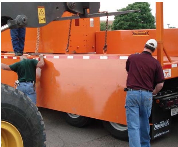
Insert tongue of axel guard through lower corner slot. Pin and clip from inside. Special 7/8" pin is provided. Check that there is adequate clearance between axel guard and tires for tires to turn freely without rubbing. Bumper can be adjusted in or out as appropriate. Trailer can be moved and run at speed with axel guard properly installed.
