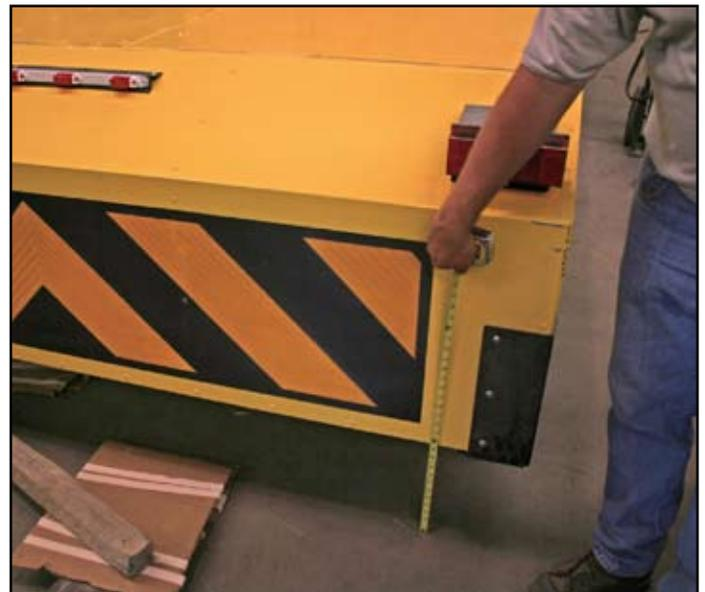
Figure 5. Measuring for cartridge height
