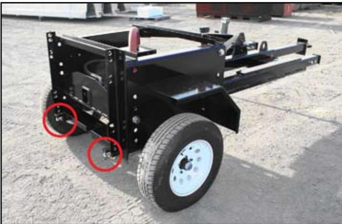
Figure 13. Loosen the jam nuts
