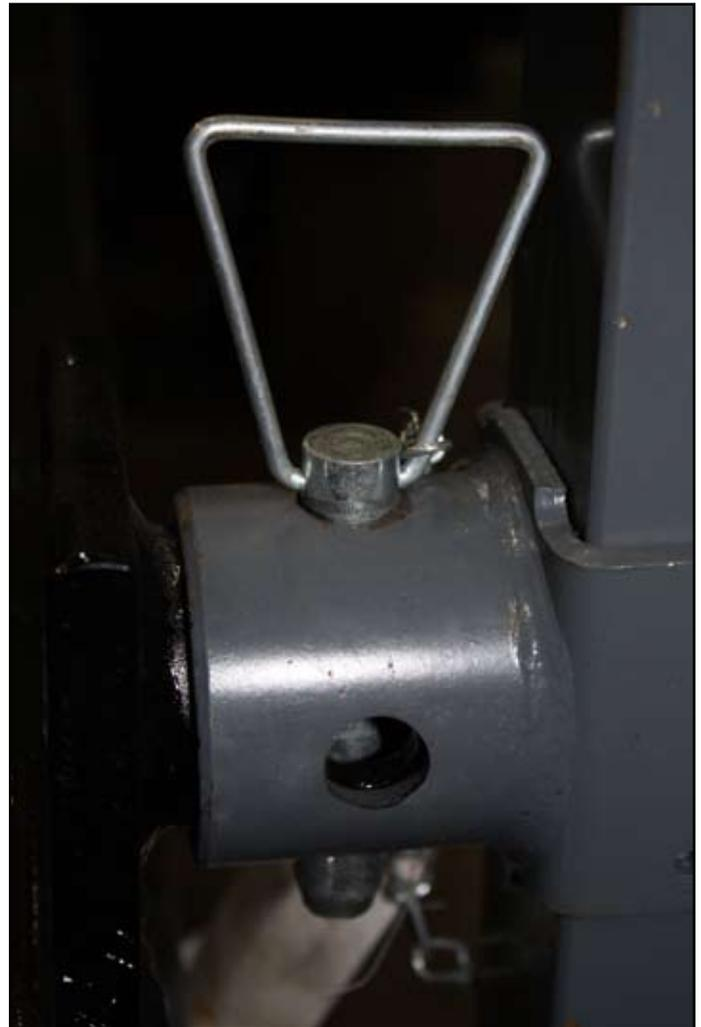
Figure 19. The jack pin is engaged
