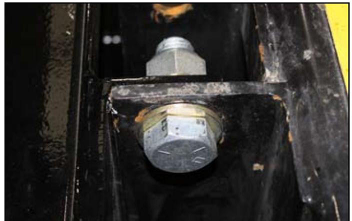
Figure 22. Check torque on mounting nuts
