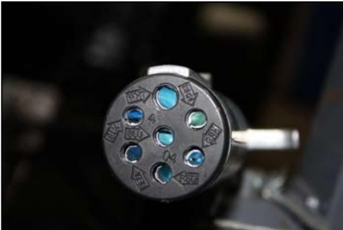
Figure 7. The 7-pin connector
