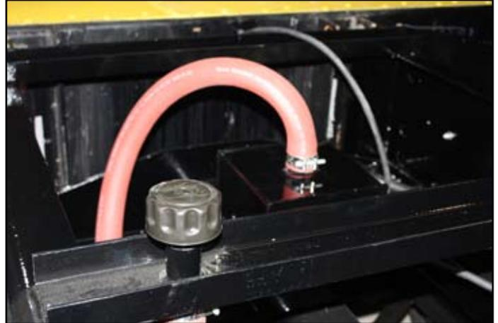
Figure 21. Check hydraulic fluid
