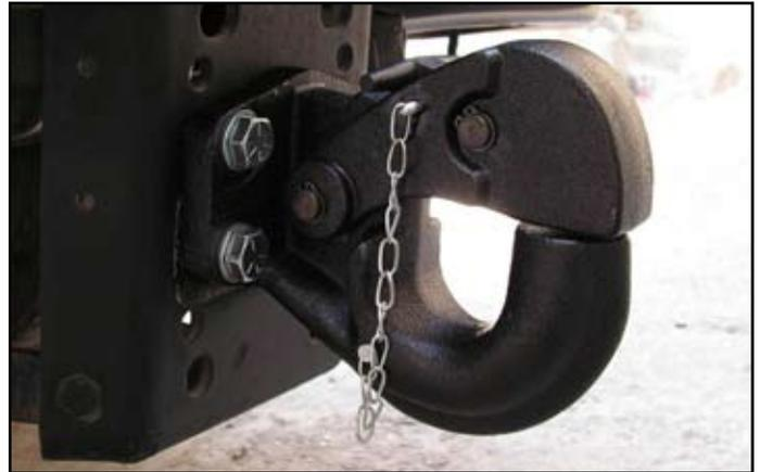
Figure 25. Check for correctly rated pintle hook
